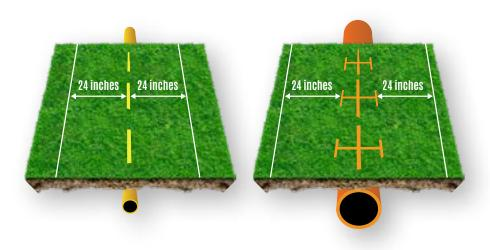
NOTE: Location markings are approximate, and the exact location may vary by up to 24 inches for gas, electric, communications, and most wastewater and potable water. (See KSA 66-1802)
